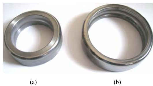
Fig. 16. Experiment results of groove ball-section ring rolling under two feed amount per revolution: (a) \Delta h=0.03mm/rev ; (b) \Delta h=0.05mm/rev .
