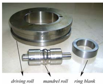
Fig. 14. Driving roll, mandrel roll and ring blank for groove-ball section ring rolling.
